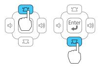
3. Press a keystone button on the projector's control panel to adjust the image shape.
